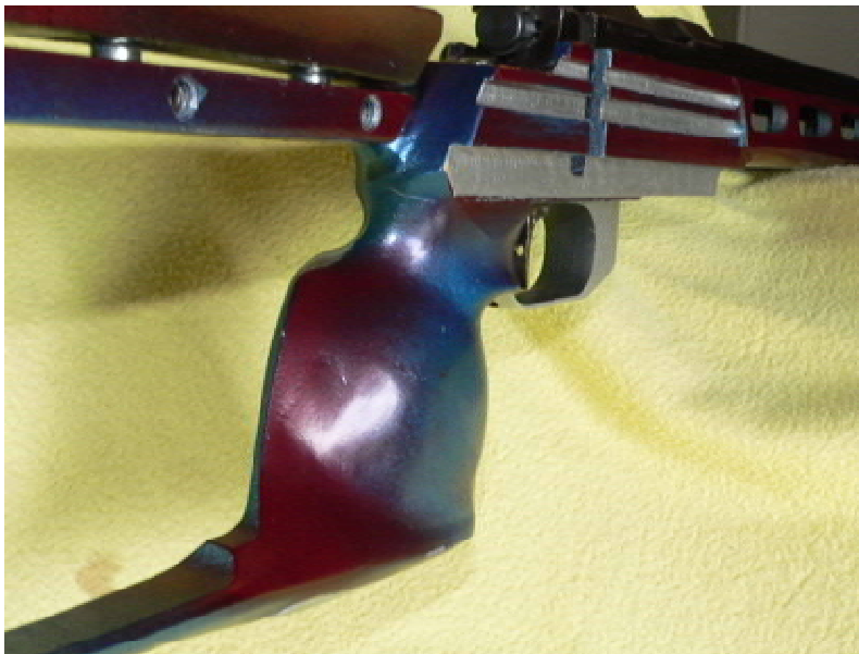
Fig 1. Showing the grip details of my own alloy stock. A great deal of attention was paid to the design which allows consistent placement of the grip and trigger finger in line with the barrel in both planes. The author believes this to be crucial in controlling the trigger release, and recoil even of a small bore rifle. The design also incorporates the placement of the thumb
